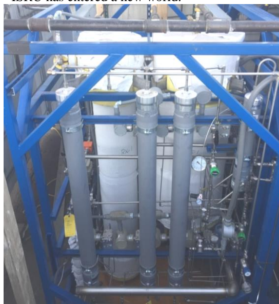
Fig. 1 Piloted Mars mission scale RWGS unit.
